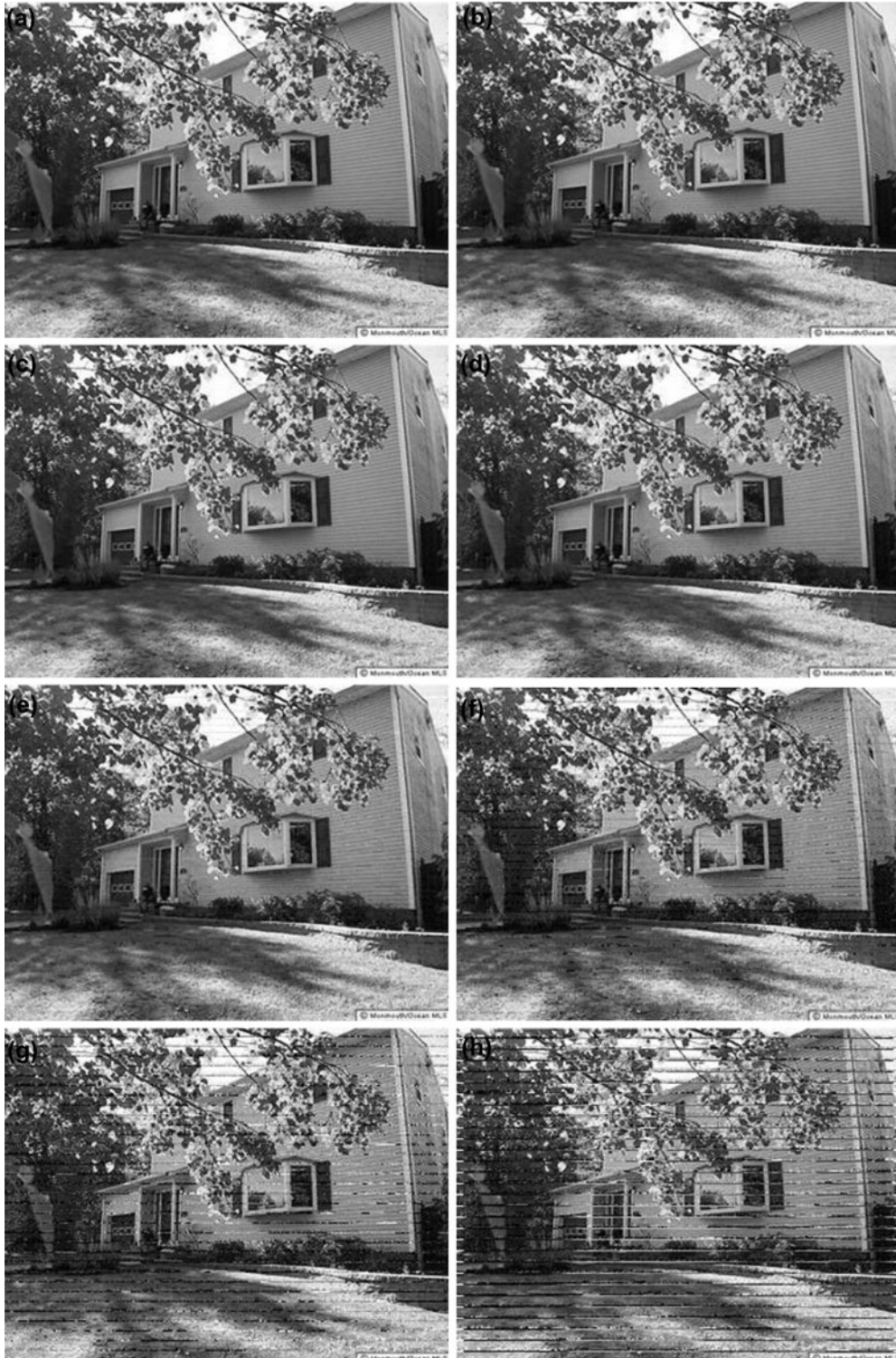
Figure 3. (a) Stego image for 2 combinations of LSBs, (b) stego image for 3 combinations of LSBs, (c) stego image for 4 combinations of LSBs, (d) stego image for 5 combinations of LSBs, (e) stego image for 6 combinations of LSBs, (f) stego image for 7 combinations of LSBs, (g) stego image for 8 combinations of LSBs, and (h) stego image for 9 combinations of LSBs.
